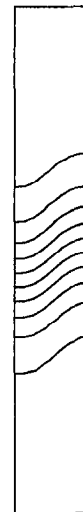
Fig. 2. Isoconcentration lines obtained from a FIDAP simulated run for the case Gr \times Sc = 360 (lateral magnification \times 10 ).
